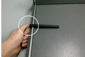
FIG 2: Position Stops, Tighten Thumbscrews
