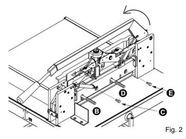
Remove the blade screws **(B)** and **(D)** and replace them with the two blade holders from the tool box. Tighten them securely.
