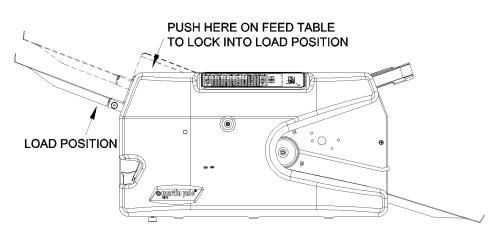
Load the paper into the Feed Table, making sure that the paper is fully within the folder, and that the leading edge of the stack is resting against the face indicated below. Once the Feed Table has been loaded with paper, the Feed Table must be unlocked, allowing the Feed Table to return to the raised position. To unlock the Feed Table, press the Feed Table Release (see illustration below).
