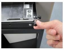
When the finish of the work piece is (A), loosen the fine adjustment knob. When the finished product is (B), tighten the fine adjustment knob.
