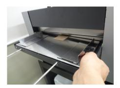
Push down on the edge of the feeder tray by hand.
