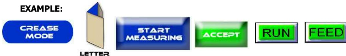
**Roll Fold:** Press the Crease Mode Button > More > Roll > Start Measuring > Physically Run a sheet through the machine for the sensor to measure > Accept > Run > Feed.
