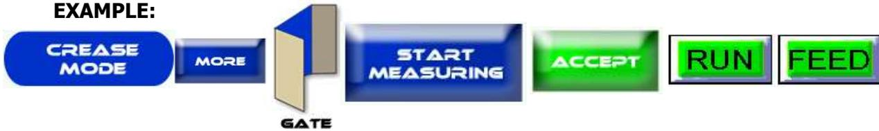
**Double Gate Fold:** Press the Crease Mode Button > More > Double Gate > Start Measuring > Physically Run a sheet through the machine for the sensor to measure > Accept > Run > Feed.
