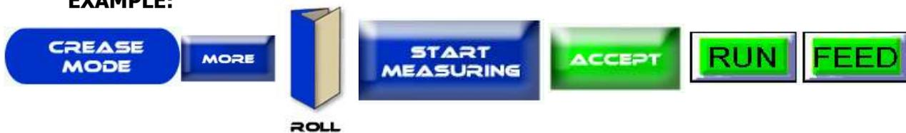
**Gate Fold:** Press the Crease Mode Button > More > Gate > Start Measuring > Physically Run a sheet through the machine for the sensor to measure > Accept > Run > Feed.
