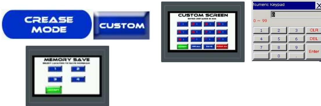
**Recalling Custom Crease Jobs:** Press the Crease Mode Button > Custom > Recall > Accept > Run > Feed.
