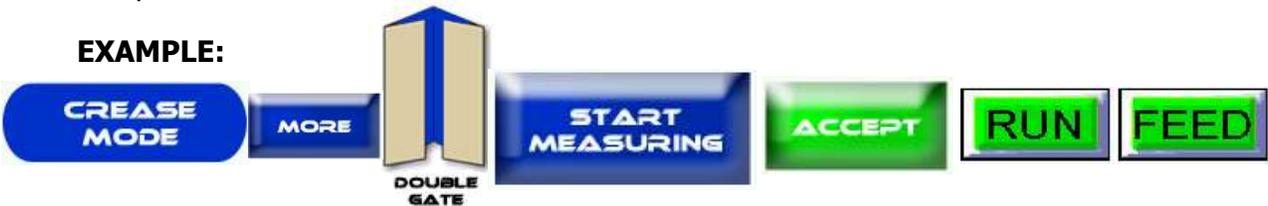
**Double Parallel Fold:** Press the Crease Mode Button > More > Double Parallel > Start Measuring > Physically Run a sheet through the machine for the sensor to measure > Accept > Run > Feed.
