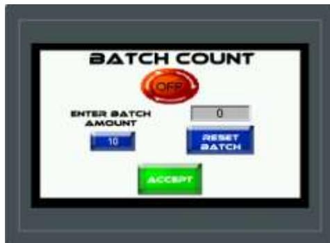
As you are running and the batch number is reached the screen will display "Batch Complete".
