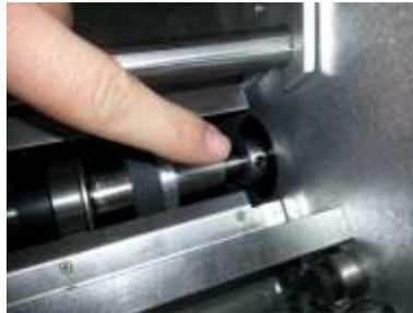
Next, remove the non-operator side cover. **DO NOT REMOVE ANY PULLEY'S!** Loosen the screws on the belt tensioned idler pulley (as shown below).
