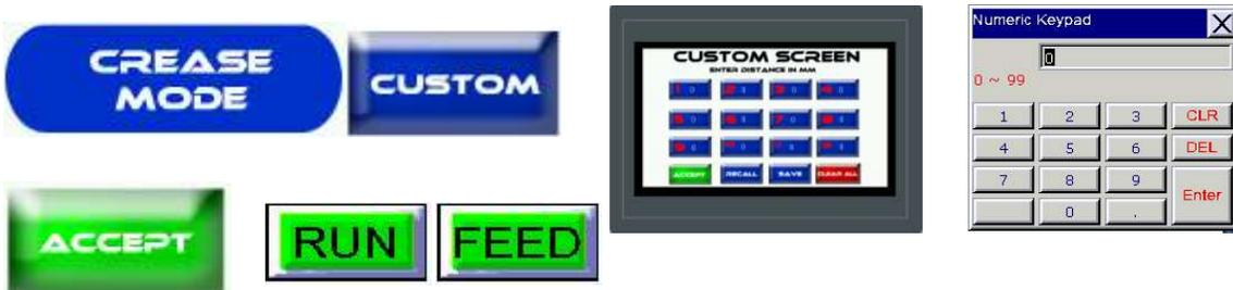
**Saving Custom Crease Jobs:** Press the Crease Mode Button > Custom > Enter In Distance For each Crease in mm > Save > Select Position to save in 1, 2, 3, or 4.
