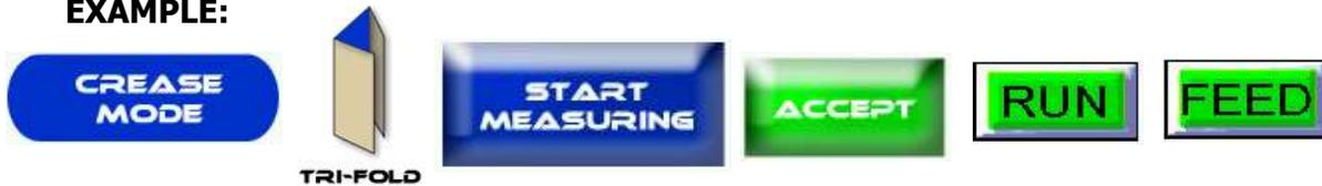
**Z-Fold:** Press the Crease Mode Button > Z-Fold > Start Measuring > Physically Run a sheet through the machine for the sensor to measure > Accept > Run > Feed.
