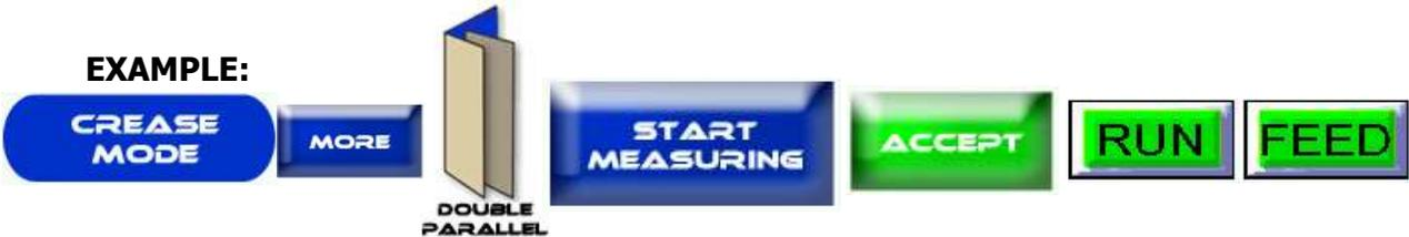
**Perfect Bind Double Hinge:** Press the Crease Mode Button > More > Perfect Binding Score > Enter The Book Thickness > Double Hinge > Start Measuring > Physically Run a sheet through the machine for the sensor to measure > Accept > Run > Feed.
