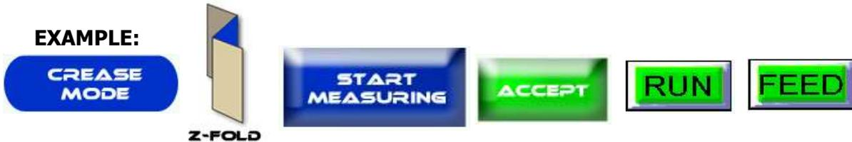
**Letter Fold:** Press the Crease Mode Button > Letter > Start Measuring > Physically Run a sheet through the machine for the sensor to measure > Accept > Run > Feed.
