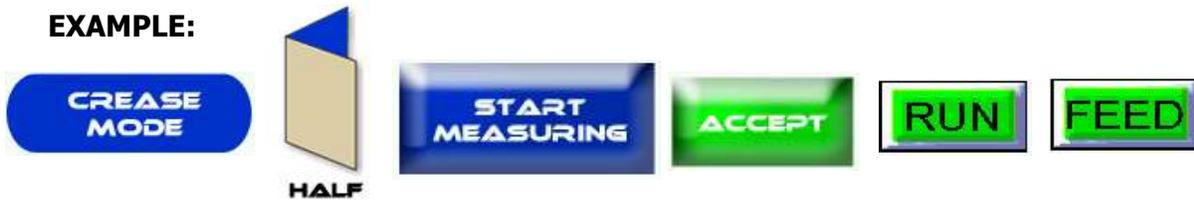
**Tri-Fold:** Press the Crease Mode Button > Tri-Fold > Start Measuring > Physically Run a sheet through the machine for the sensor to measure > Accept > Run > Feed.
